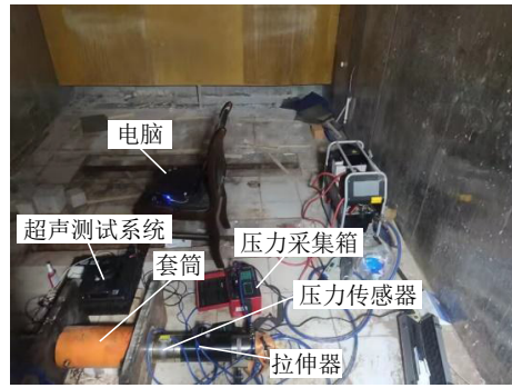
图 3 环境试验箱内超声测试设备照片 Fig.3 Photo of ultrasonic testing equipment in environmental laboratory
